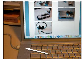
Internal omni-directional microphone (eg; located under left speaker grille)
