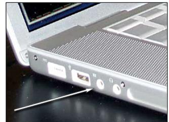
Line in ~ mini-jack stereo input jack for a stereo microphone
